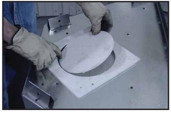
Figure 9.2 Remove the center insulation plug.
